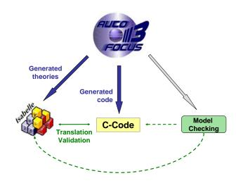
Fig. 2. Generation Tool Chain and Validation Mechanisms
